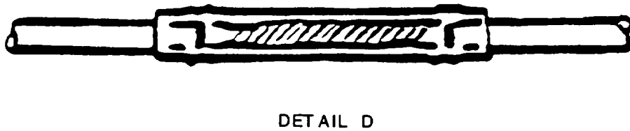
Figure 4-3. Solder Method to Repair Wires.
